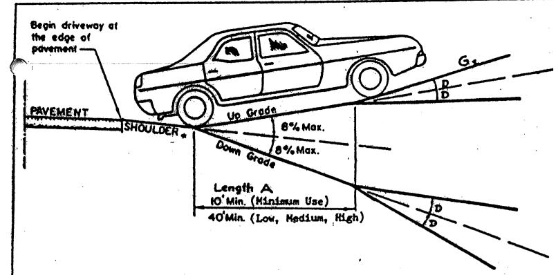
"The shoulder slope usually varies from i"/ft.(4) to 3/4"/ft.(4). However, the shoulder slope should be maintained when constructing the driveway.
